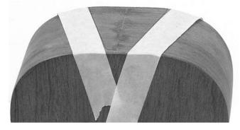
Now that the heel fits the body, align the fingerboard with the centerline on the top. Make a pencil outline of the heel on the side of the body. Remove the neck and mask the gluing area with masking tape. The tape will guide you in positioning the neck when gluing it.
