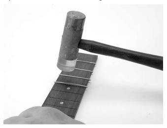
As each fret is seated, nip the overhanging ends close to the sides of the fretboard (approximately 1/64"). Leaving a little overhand helps you avoid marring the wood. Fret nippers are ideal for this job, and provide a clean, flush cut. Wire cutters will do if you don't have fret nippers.
