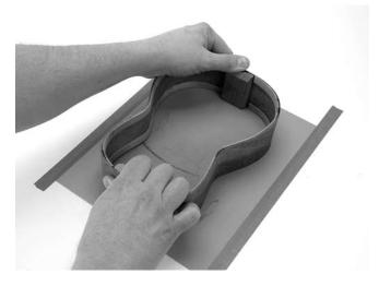
When the back edges are sanded, turn the body over and level-sand the top in the same way. Watch to make sure you keep things level, so you have equal depth on both the left and right sides.
