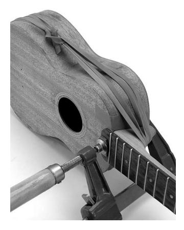
Dry-clamp the neck using a clamp on the fingerboard where it overlaps the body. Use scrap wood to protect the fingerboard and the back. Then wrap rubber bands around the body and neck heel. When you're ready to glue, spread Titebond onto the neck and fingerboard extension where it contacts the body. Reclamp and allow to dry for at least 3 hours.
