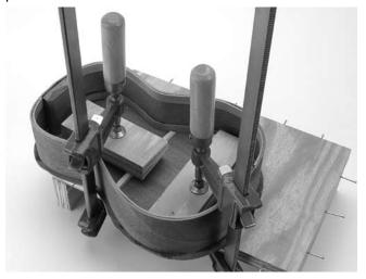
When you're comfortable with your clamping setup, use Titebond glue and clamp the braces and bridge plate. Allow 3 hours to dry.
