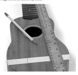
Position the bridge with the saddle slot centered over this pencil line, and place a piece of masking tape along the bottom edge of the bridge. Center the bridge by extending straightedges from both sides of the fingerboard. When it's centered, use masking tape to mark the left and right ends of the bridge.
