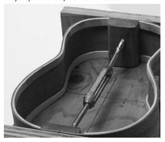
Align the sides with the profile on the base of the jig. It may be necessary to drive a few finishing nails into the jig to hold the sides in a good symmetrical shape. Double-check your alignment with the centerline.
