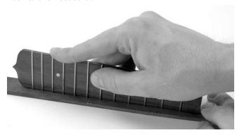
Next, hold the file at an angle and put a beveled shape onto the fret ends. An angle of 60-degrees is about right, but the steepness of this bevel is a matter of personal preference.
