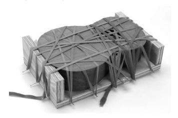
When you're comfortable with this process, untie the bands and spread a thin line of Titebond glue along the top edge of the lining. Center the top on the body again, making sure you have a bit of overhang all around edges. Use the rubber
